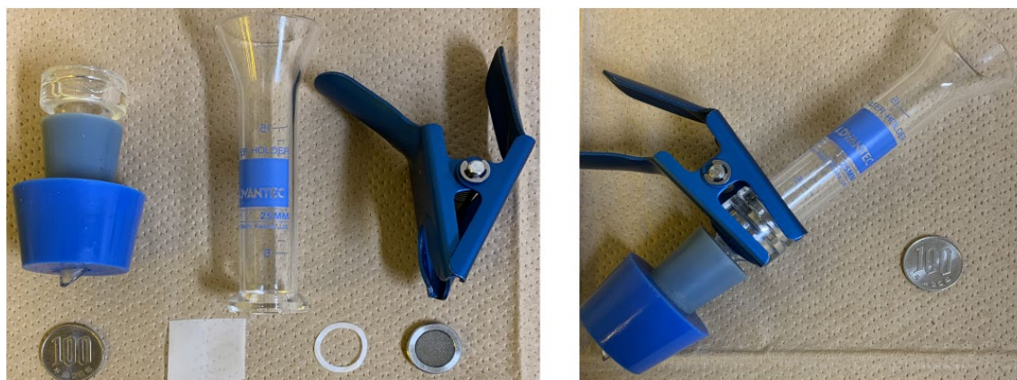
Figure A.11 Images of filter device with each part (left) and assemble (right)
