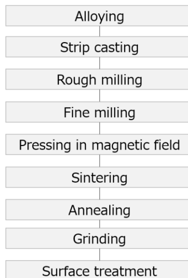
Figure 1-2 Typical Nd-Fe-B magnet manufacturing process.
