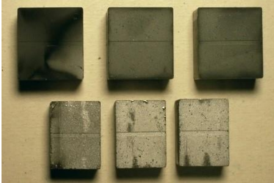
Figure 4-5 Image of sintered magnet prepared from magnet powder with (Upper) and without (Lower) PVA.
