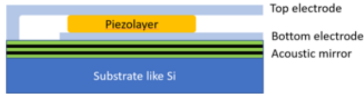
Figure 1.14: A schematic of FBAR: solidly mounted (SMR). Reproduced from Wikipedia under the Creative Commons Attribution-Share Alike 4.0 International License
