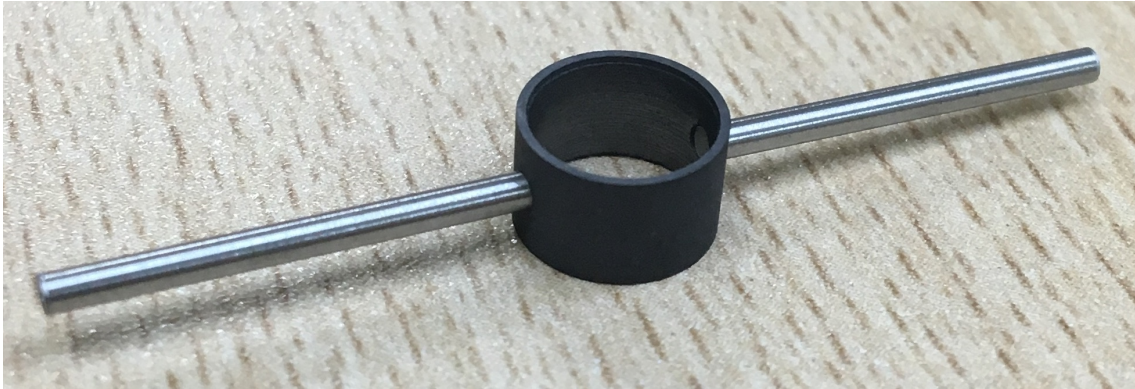
Fig. S7-1. The tested cylindrical shape graphite ring heater with the wall thickness of 0.5 mm.
