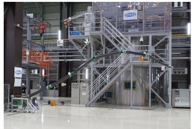
Fig. 1 Super Dragon: a 10 m-long coupled tendon-driven robot arm.
