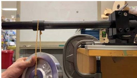
Fig.3 Fix CFRP pipe to OTA's output axis
