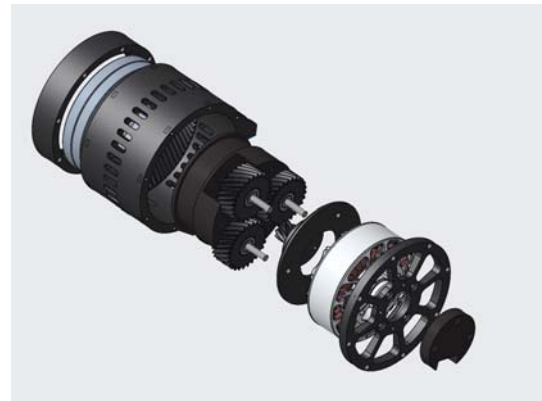
Fig.1 Overall structure of OTA
