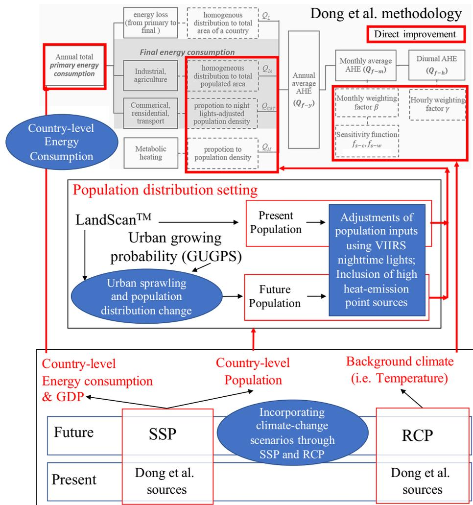
**Fig. 1** Workflow of AH4GUC construction. AH4GUC directly influences the components bounded by red boxes in the methodology of Dong *et al.*<sup>10</sup>, region in grey (figure used with permission).
