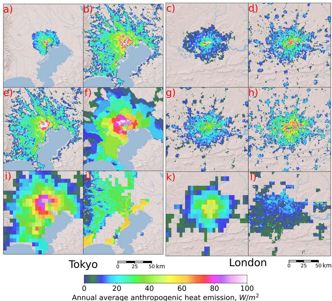
**Fig. 2** Comparison of anthropogenic heat emission datasets for Tokyo and London. “Bottom-up” approaches by (a) Moriawaki *et al.*<sup>21</sup> and (c) Iamarino *et al.*<sup>22</sup> for Tokyo and London, respectively; (b,d) AH4GUC; (e,g) DONG<sup>10</sup>; (f,h) PF-AHF<sup>9</sup>; (i,k) FL<sup>2</sup>; (j,l) AH-DMSP<sup>8</sup>. Values lower than 5 W/m<sup>2</sup> are masked.
