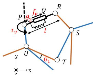
Fig.11 Definition of symbols used in kineto-static analysis
