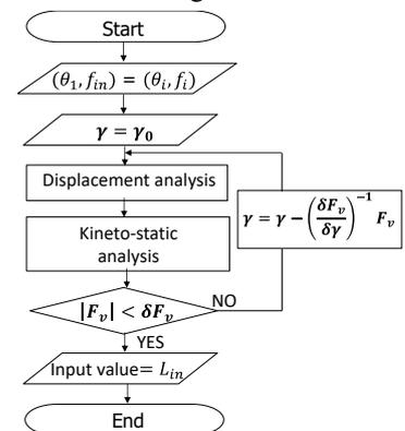
Fig.12 Flowchart of kineto-static analysis
