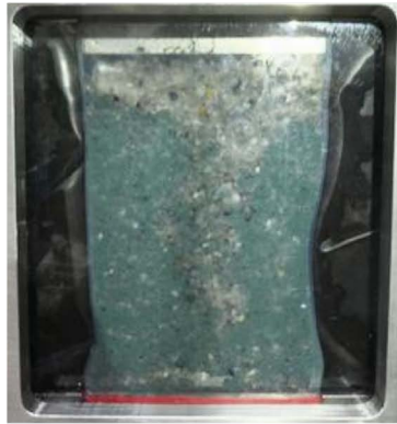
(b) During seepage test
