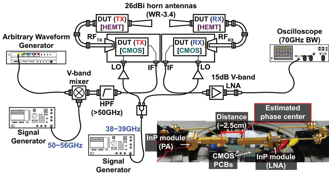
Figure 4.30: Hybrid transceiver measurement setup. (© 2021 IEICE)
