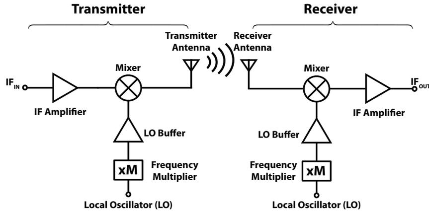
Figure 1.4: Generic architecture for the 300GHz-band transceiver.
