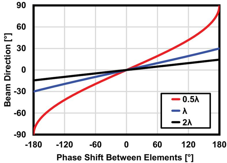
Figure 2.4: Beam steering range for different antenna pitch lengths.
