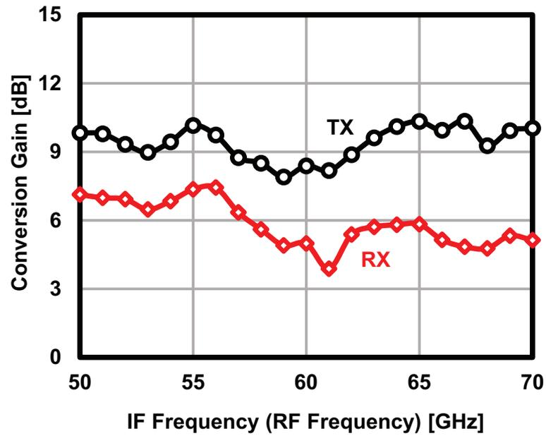
Figure 4.16: Measured TX and RX conversion gain values.
