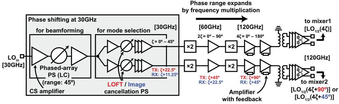
Figure 5.7: LO chain block diagram.
