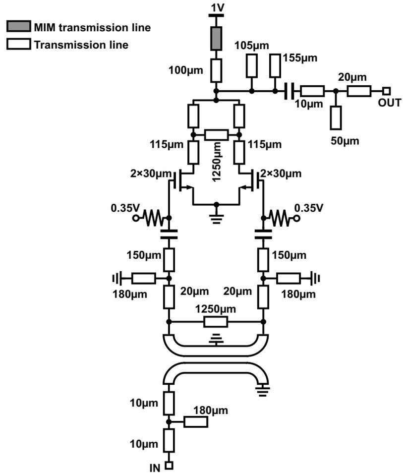
Figure 3.22: Proposed push-push frequency doubler detailed schematic.
