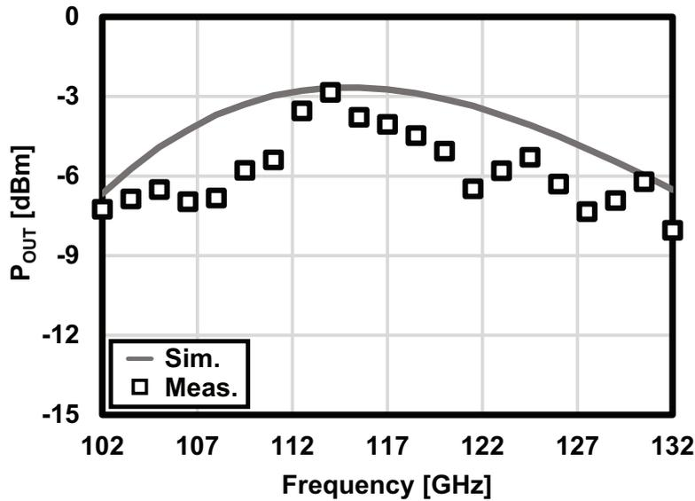
Figure 3.12: Tripler measured and simulated output power. (input power = 10dBm)
