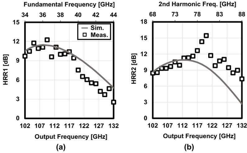
Figure 3.13: Tripler measured and simulated fundamental rejection ratio. (input power = 10dBm)
