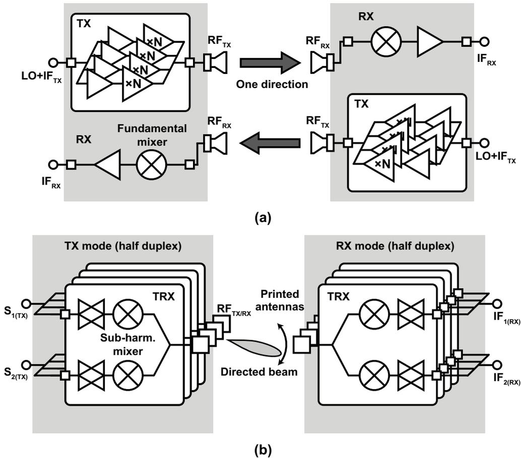
Figure 5.1: (a) Conventional sub-THz transceiver (b) Proposed transceiver with bi-directional architecture and beamforming.
