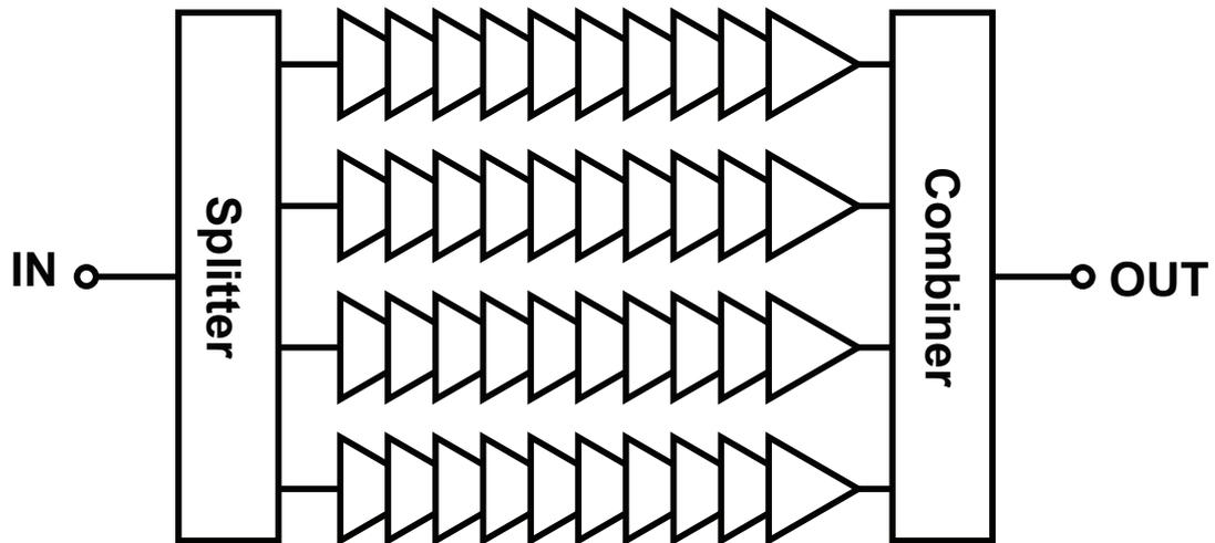
Figure 6.3: Possible CMOS 300GHz-band power amplifier structure.
