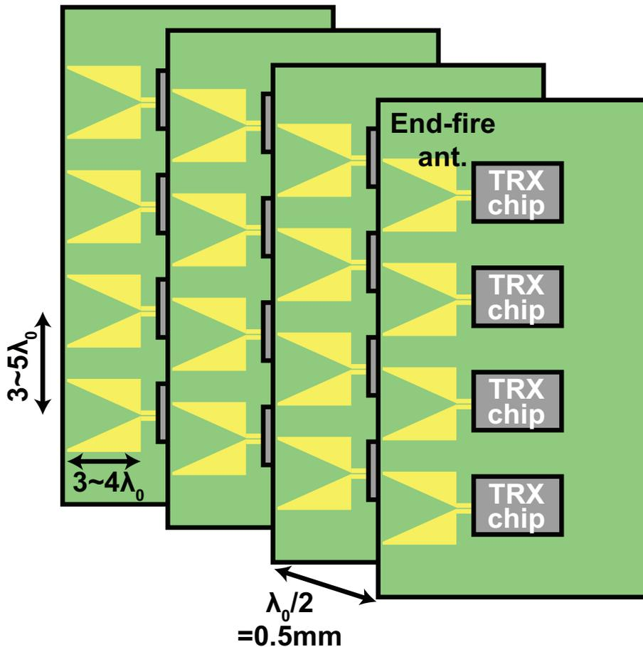
Figure 6.4: Two-dimensional array implementation using stacked PCBs.
