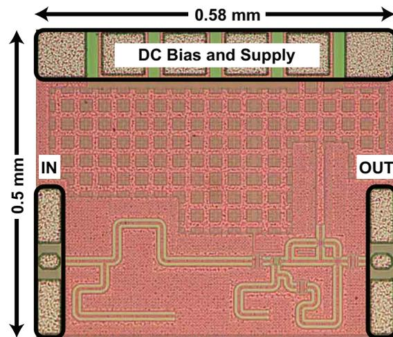
Figure 3.10: Frequency tripler micrograph. (© 2021 IEICE)
