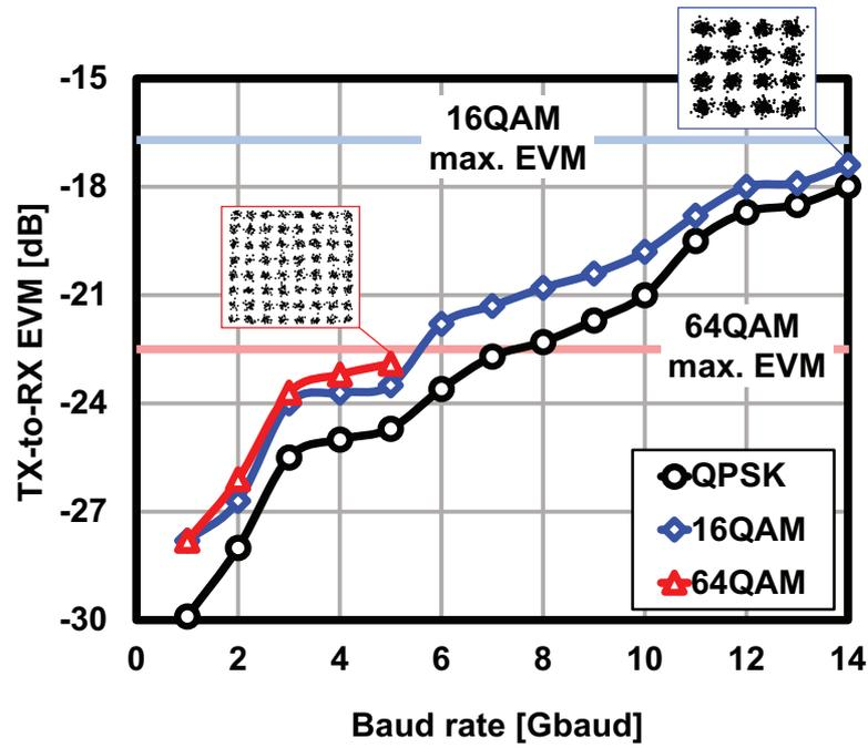
Figure 4.31: Hybrid transceiver measured EVM vs baud rate.
