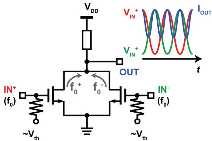
Figure 3.19: Conventional push-push frequency doubler and its operation.
