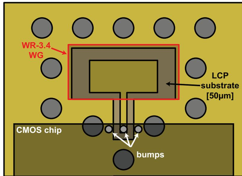
Figure 5.24: CMOS-to-PCB transition design for PCB evaluation board.
