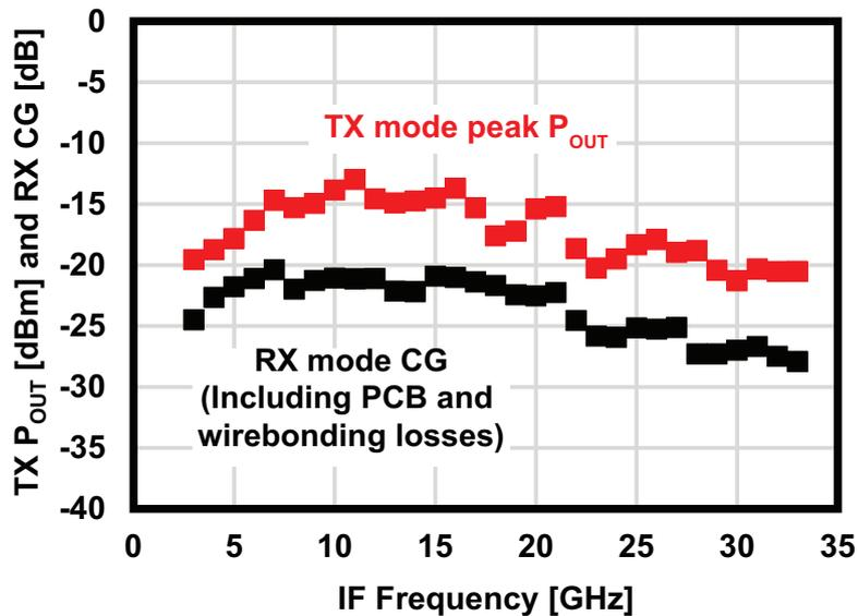
Figure 5.27: Measured TX mode output power and RX mode conversion gain.
