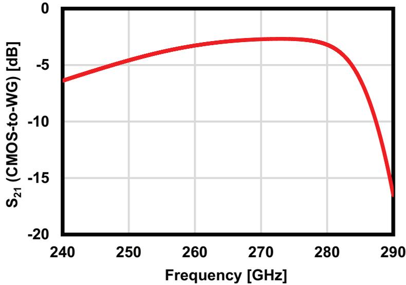
Figure 5.26: Simulated loss of the CMOS-to-WG transition.
