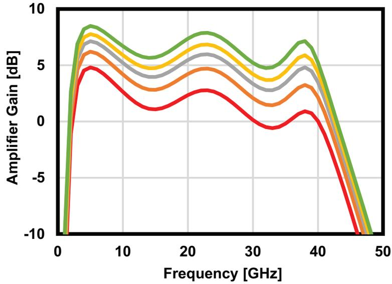
Figure 5.16: IF amplifier simulated gain for several voltages.
