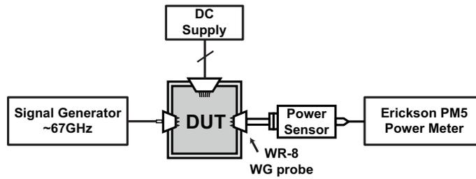
Figure 3.11: Measurement setup.
