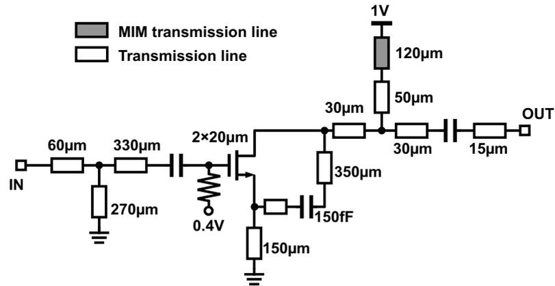
Figure 3.9: Proposed frequency tripler circuit schematic.
