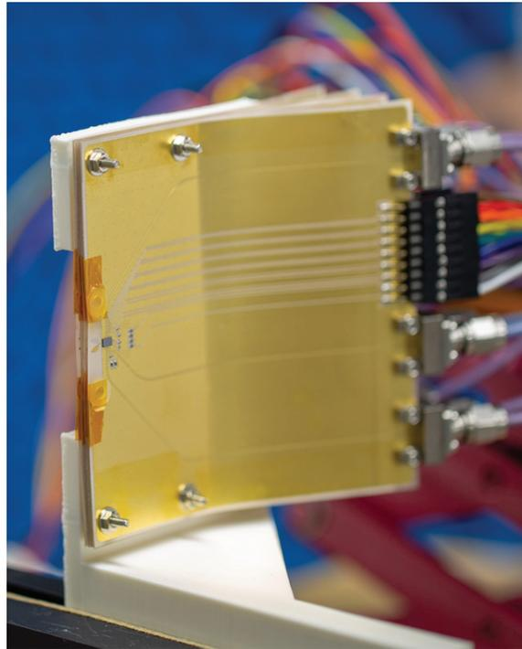
Figure 5.23: A photograph of the implemented 4-element phased-array.
