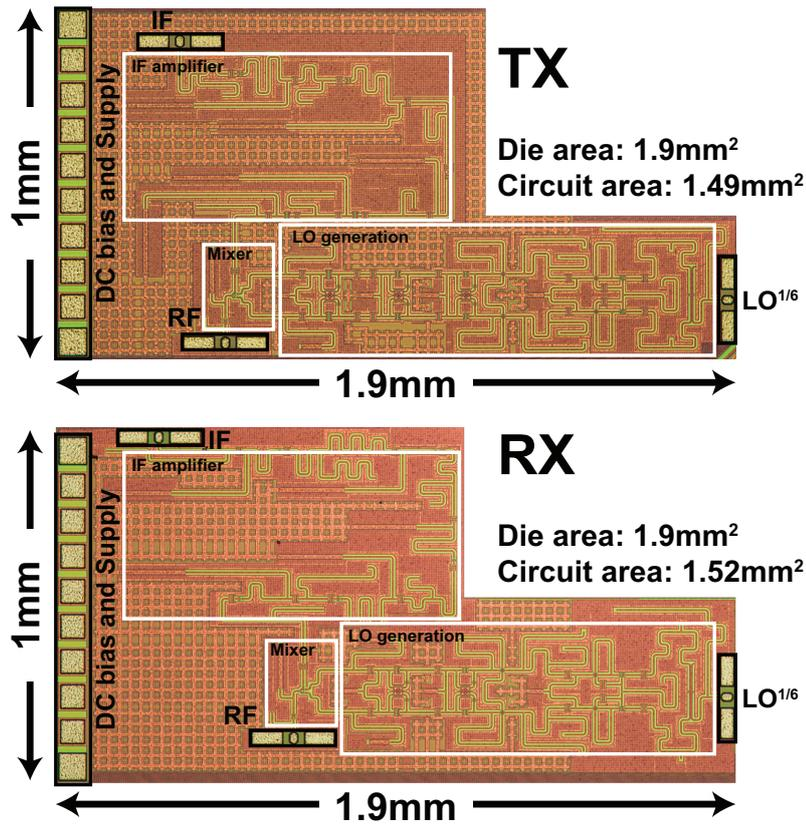
Figure 4.15: CMOS TX and RX chip photos. (© 2020 IEEE)
