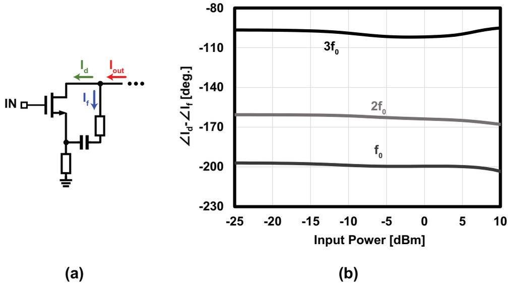
Figure 3.7: Frequency tripler simulated operation: (a) The simulated currents, (b) The simulated phase difference between the drain and the feedback currents. ( $f_0=38\text{GHz}$ ,  $P_{\text{IN}}=10\text{dBm}$ )
