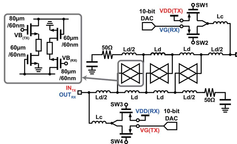
Figure 5.15: Bi-directional distributed variable-gain IF amplifier schematic.
