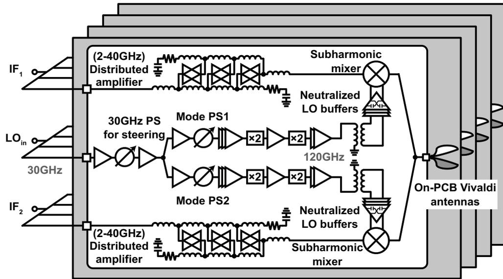
Figure 5.2: Bi-directional 300GHz-band phased-array transceiver architecture.
