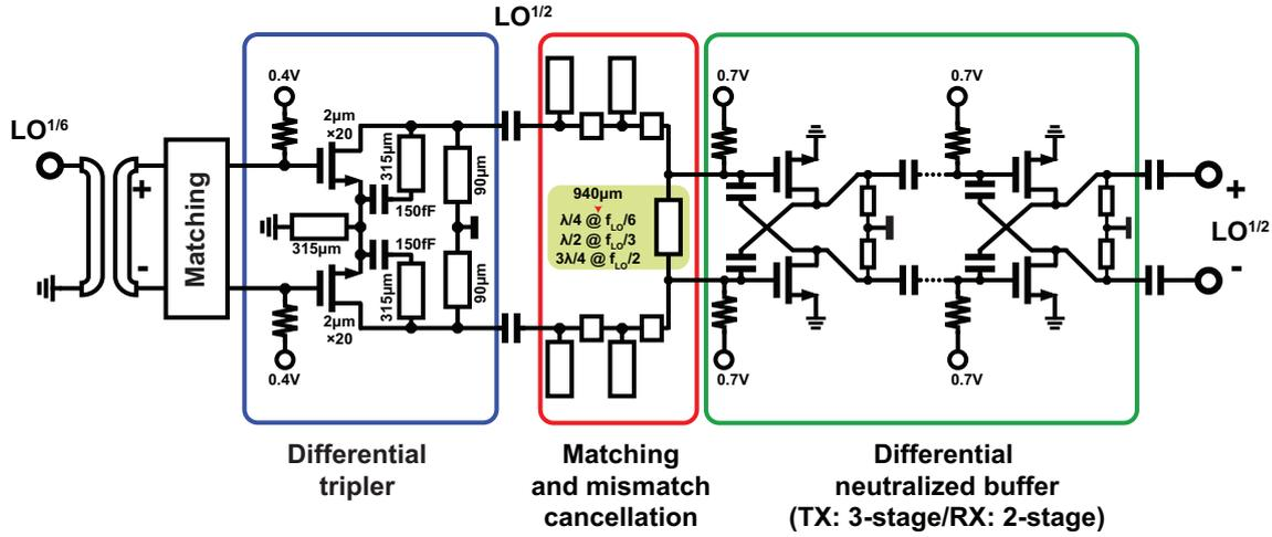
Figure 4.9: LO chain circuit schematic.
