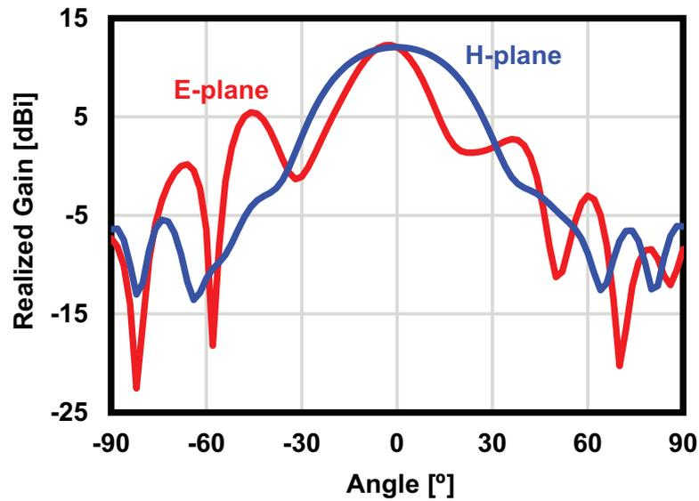
Figure 5.21: Vivaldi antenna simulated realized gain in the E-plane and the H-plane (including the connection to CMOS).
