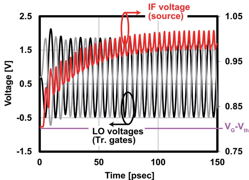
Figure 4.5: Transient simulation of the source voltage.
