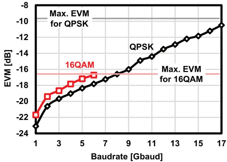
Figure 4.24: Measured EVM versus baud rate for 1cm distance.
