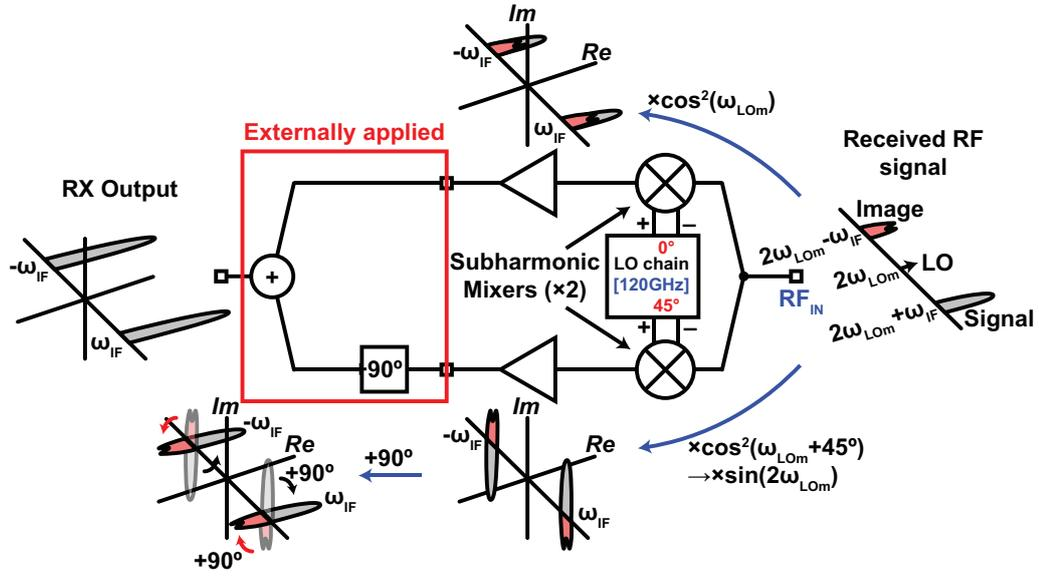
Figure 5.6: The operation of the Hartley receiving mode.
