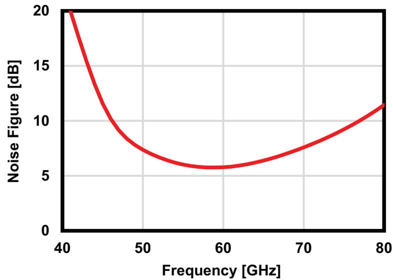
Figure 4.13: Simulated RX IF amplifier noise figure.
