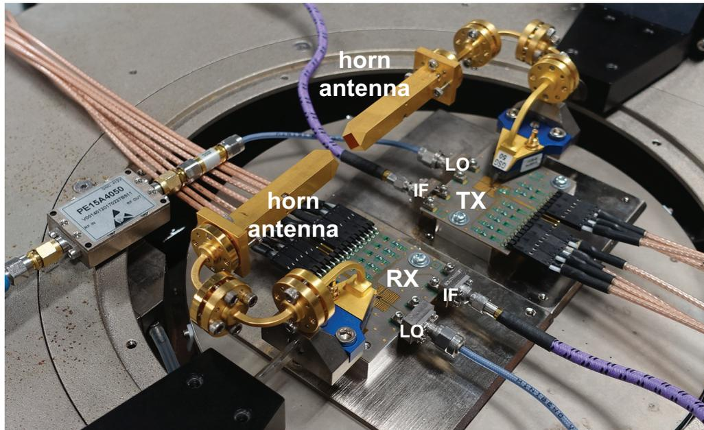
Figure 4.20: CMOS transceiver measurement setup photo. (© 2020 IEEE)
