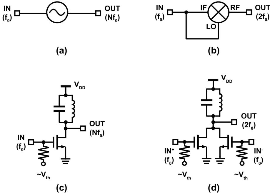
Figure 3.1: Conventional frequency multiplier topologies: (a) Injection-lock-based, (b) Mixer-based, (c) Device nonlinearity-based, and (d) Push-push-based.
