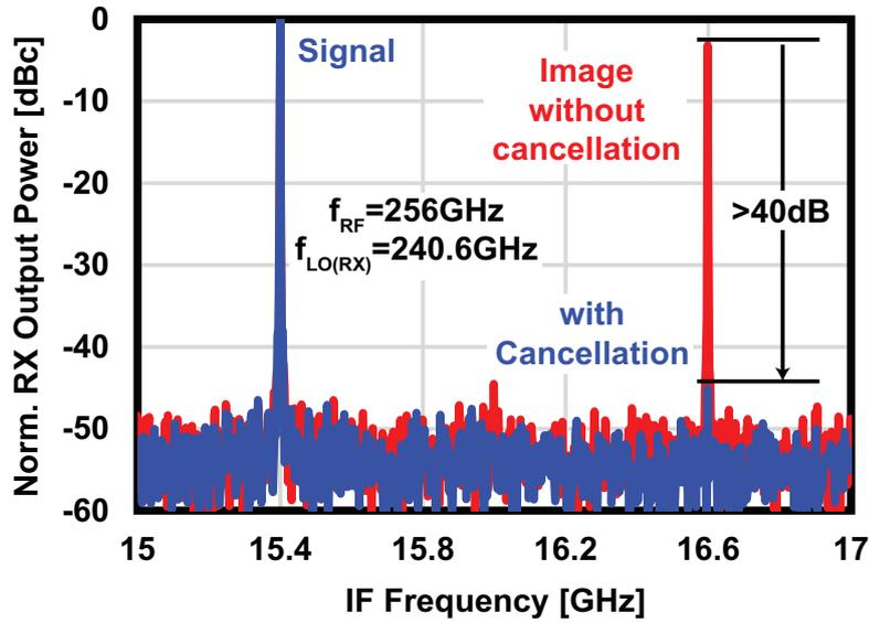
Figure 5.30: Measured image rejection of RX Hartley mode.
