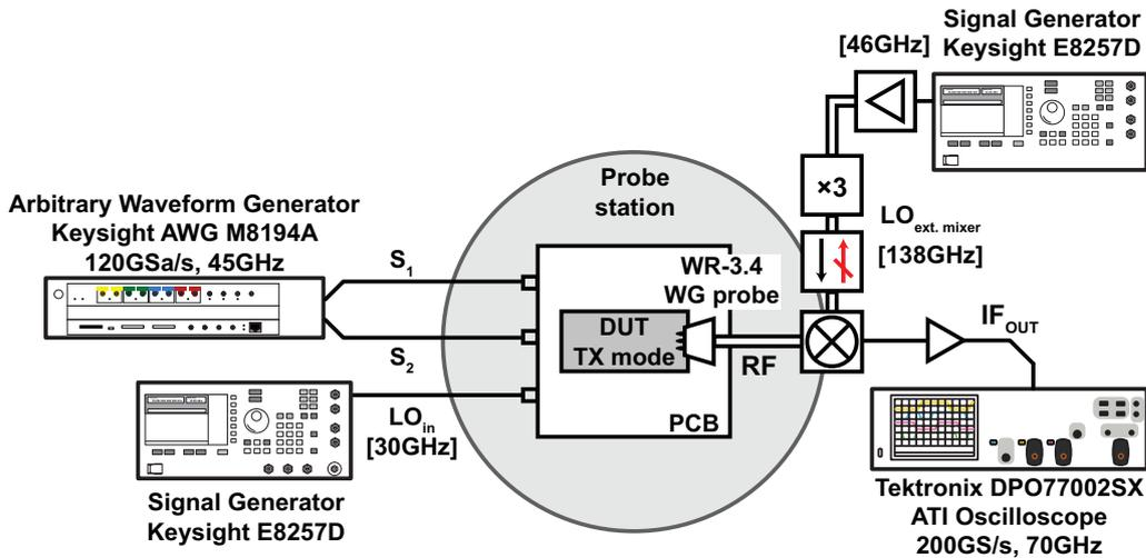
Figure 5.31: Measurement setup for TX mode EVM.
