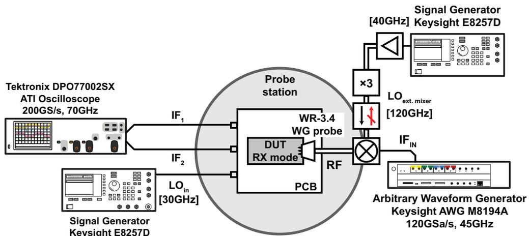
Figure 5.32: Measurement setup for RX mode EVM.
