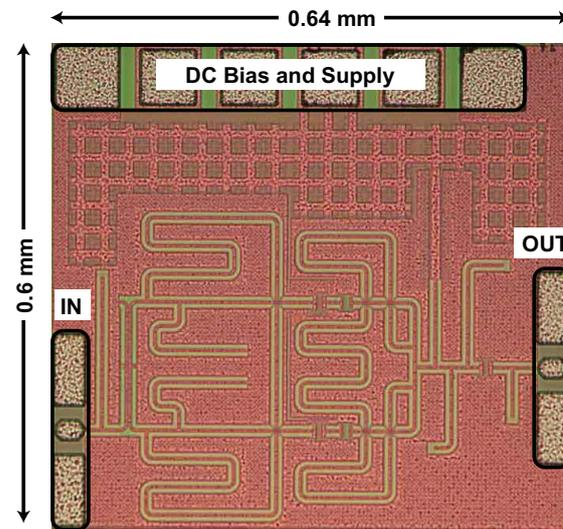
Figure 3.23: Proposed push-push frequency doubler micrograph. (© 2021 IEICE)
