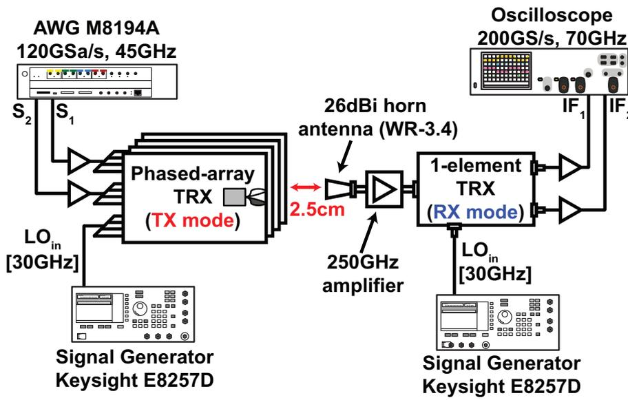
Figure 5.36: Array pattern measurement setup block diagram.
