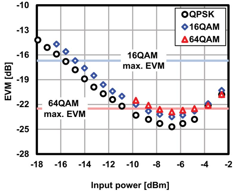
Figure 4.32: Hybrid transceiver measured EVM vs input power.
