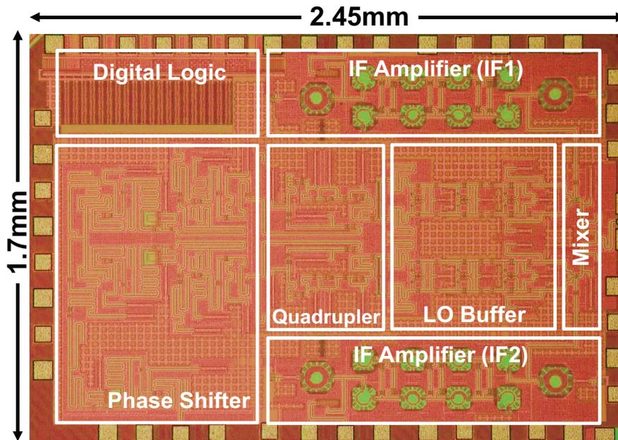
Figure 5.17: The die micrograph. (© 2021 IEEE)
