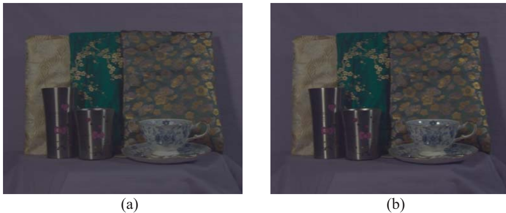
Figure 4.8 (a) Saturated versus (b) restored RGB images. Note that the color range in the (a) saturated image was adjusted such that the color of the non-saturated region appears the same in both images.
