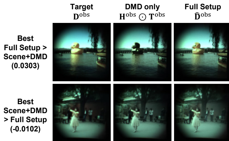
Figure 6.9: Results that the full setup is most superior to the DMD-only setup, and vice versa in the basic-GT condition. The values under the row legends are the differences of LPIPS between the scene+DMD and the full setup.
