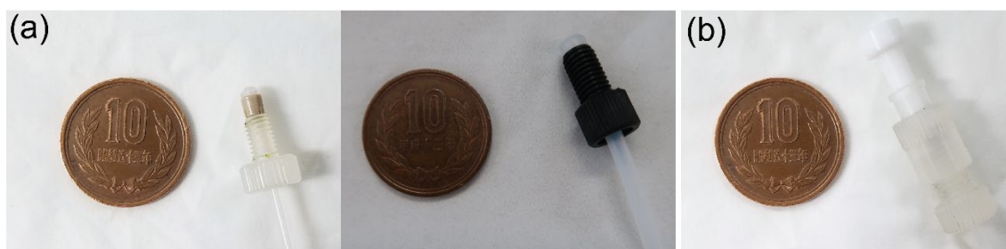
Fig. A.8 HPLC connectors for linking the (a) holder and (b) syringes.
