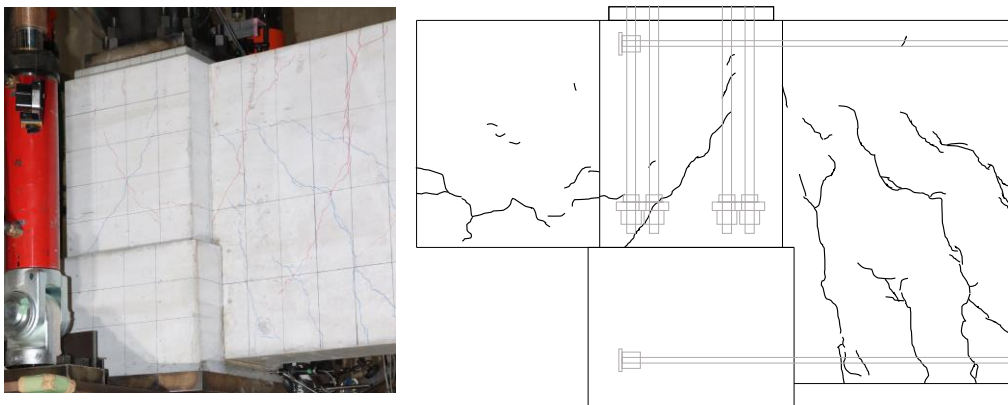
Figure 2-13 Concrete breakout failure cracks occurred in specimen B16-590-20d when R = +1/75
