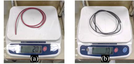
Fig.5 Power line (a: AWG16 copper, b: Ø2 mm Aluminum)
