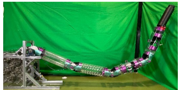
Fig.1 Coupled tendon-driven manipulator 'Mini 3D CT-Arm' with the proposed end-effector
