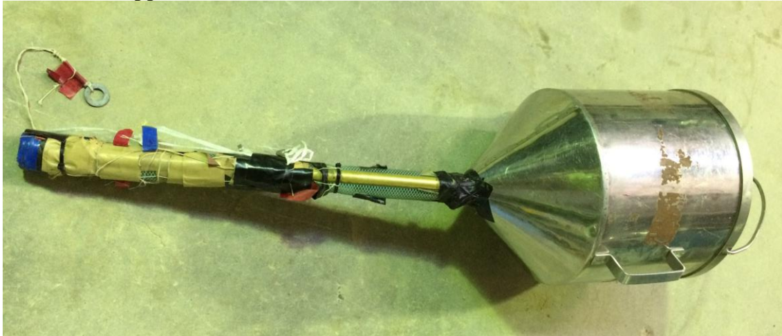
Figure 3.38 Sand hopper used in the centrifuge modelling of dry Toyoura sand at required density
