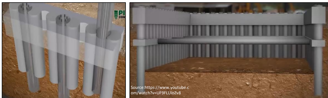
(a) Installation of male and female piles
