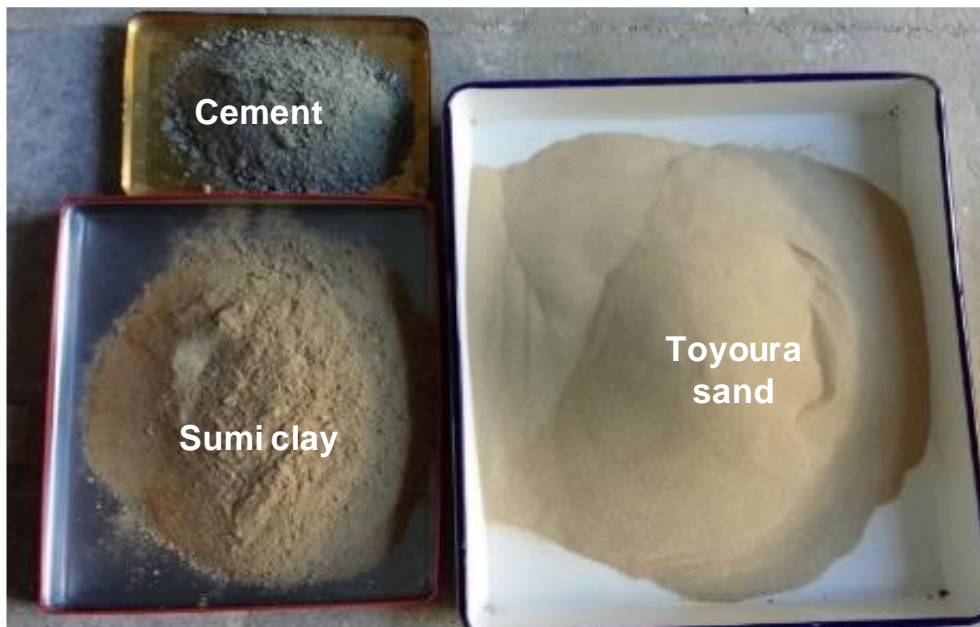
Figure 3.3 Material used for the modelling of artificial soft rock
