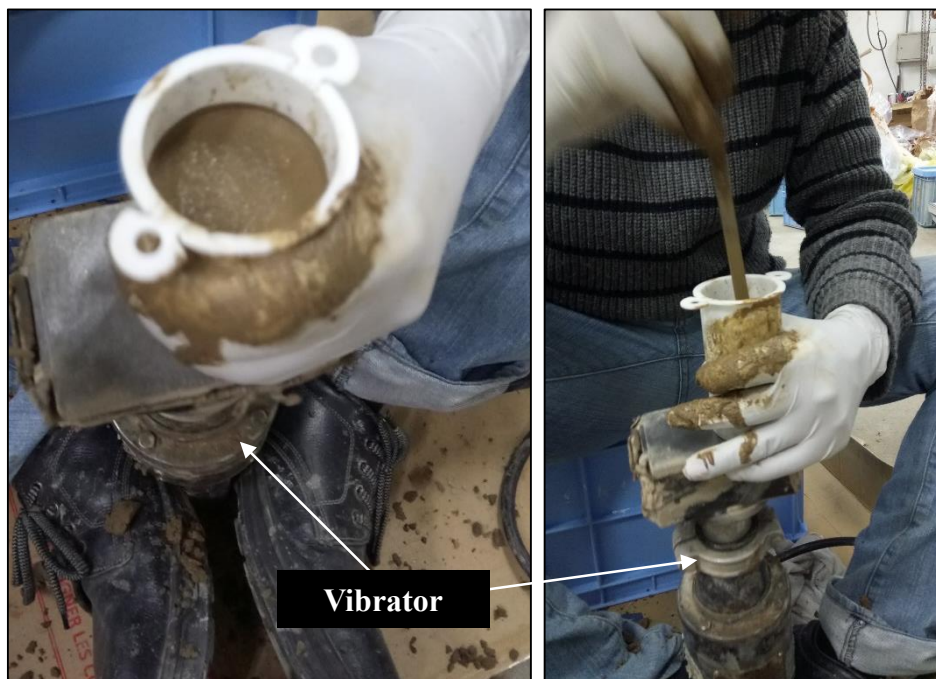
Figure 3.9 Preparation of moulded specimens
