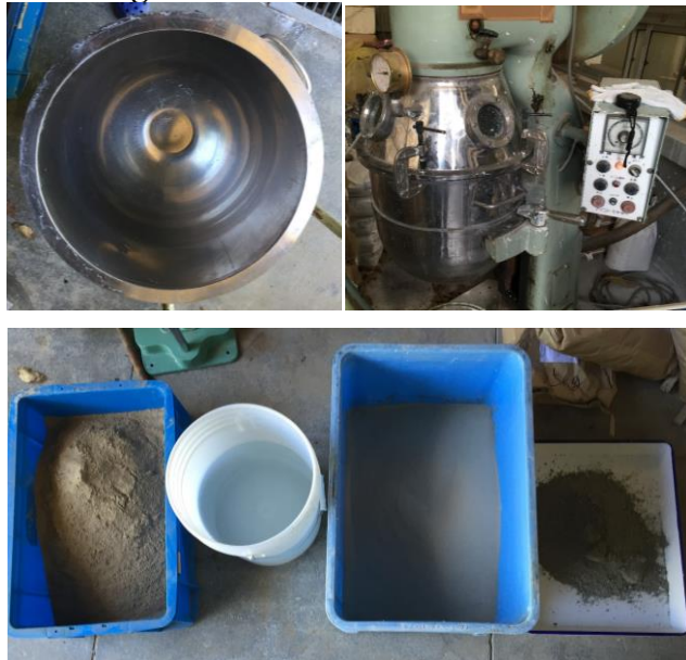
Figure 3.29 Mixing mould and constituents of one batch mix (approximately 28L)
