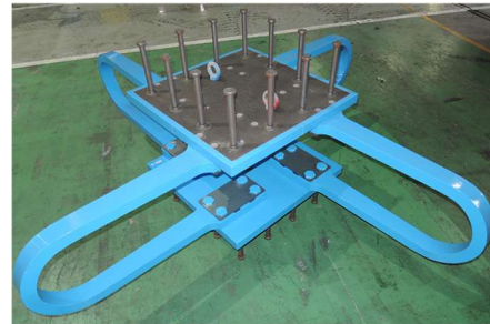
(b). U-shaped steel damper [1-18]
