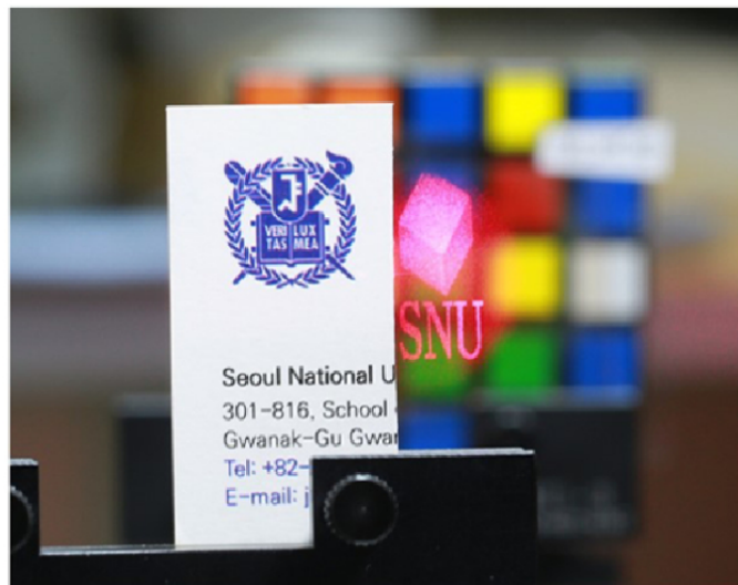
Figure 2.6: Background combination with the HOE screen to show its potential use as part of an AR system. Source: [38]
