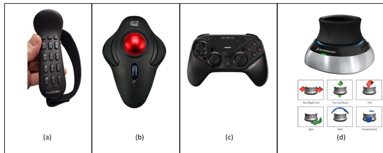
Figure 2.7: Some traditional 3D input hardware devices to achieve 3D interaction. (a) A 12-key chord keyboard. (b) A mouse with a trackball. (c) Joysticks on a video game controller. (d) Desktop 6-degrees of freedom input device with some of its gestures indicated below. Source: [36]
