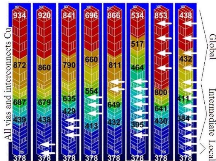
Fig. 1.9 Interconnect temperature [K] using different proportion of CNT via layer [48]
