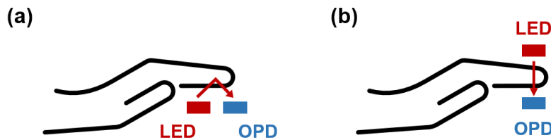
Fig. 5.1. Schematic illustration of (a) reflection type and (b) transmission type PPG sensor.
