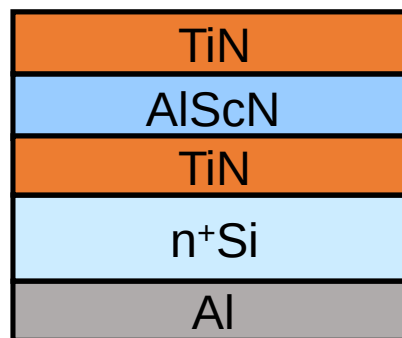
Figure 3.2 A schematic illustration of the fabricated AlScN MIM capacitor.
