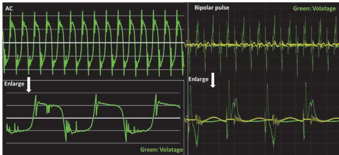
Figure 3–3. Voltage and current waveform of plasma generated by AC 50 Hz (left) and bipolar pulse with 20 kHz (right)
