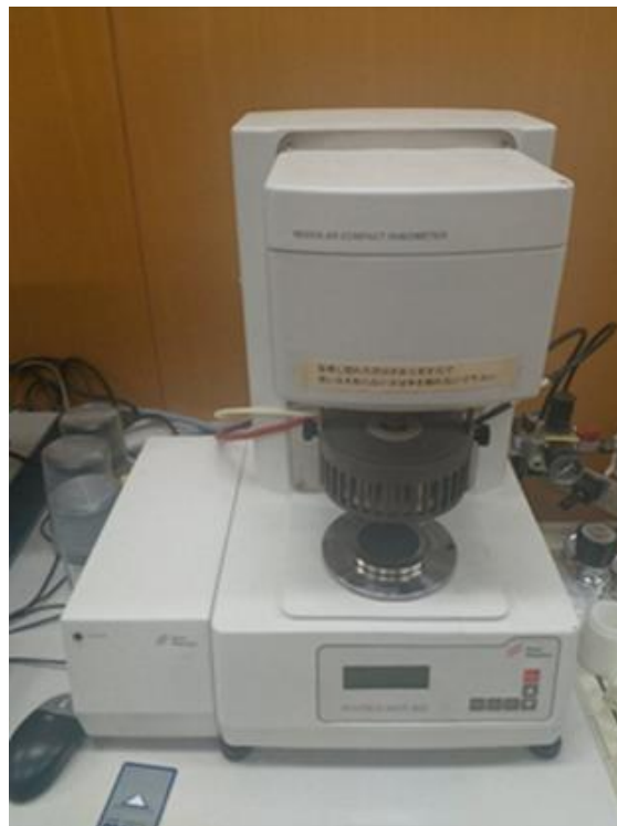
Figure 2-4. Anton-Paar MCR 300 rheometer for the steady shear viscosity measurement.
