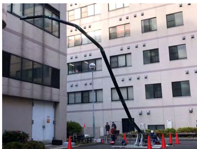
Fig.1 10-meter coupled tendon-driven super-long articulated arm for decommissioning of Fukushima Daiichi Nuclear Power Plant "Super Dragon".
