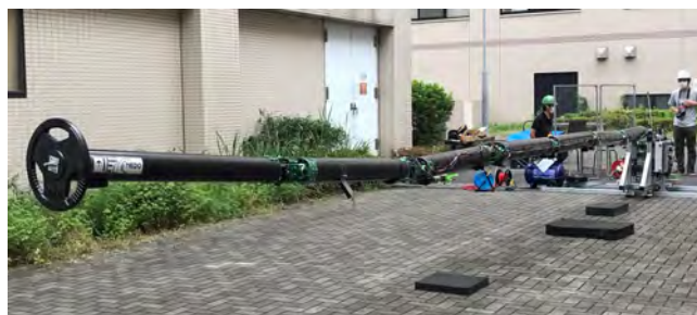
Fig.2 Power consumption testing of Super Dragon in horizontal posture with 10 kg payload.
