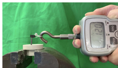
Fig.3 Experimental apparatus for measurement of output pin tilt
