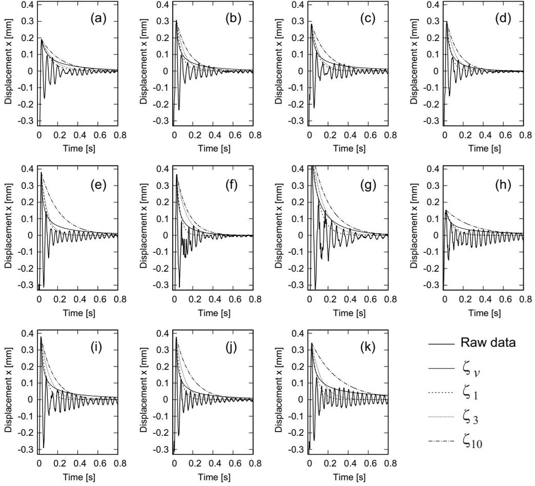
Fig. 5. Experimental results and damping ratio characteristics  $\zeta_1$ ,  $\zeta_3$  and  $\zeta_{10}$  a: A2017, b: A5052, c: A7075, d: Armigo Hard, e: MC901 nylon, f: Onyx-FR, g: Onyx-N, h: POM, i: POTICON, j: FELCARBO, k: UNILATE
