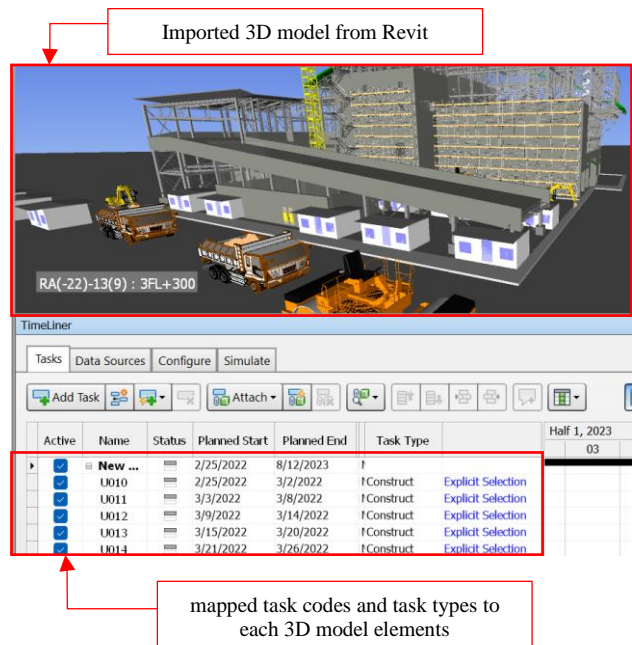
Figure 7. The imported 3D model from Revit to Navisworks with mapped task codes and task types.
