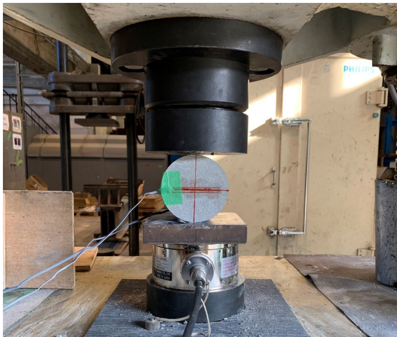
Figure 51 Split-tensile test experimental setup.
