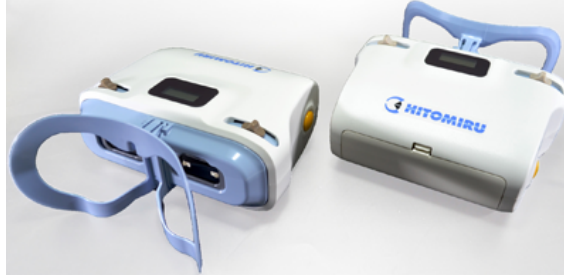
Fig. 1. Equipment to observe pupillary changes
