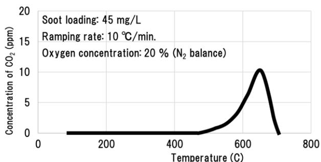
Fig.10 Temperature program oxidation of soot trapped on the TWC particles membrane filter
