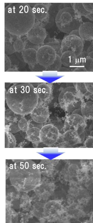
Fig.9 Time-lapse SEM images of surface views during soot deposition on the surface of TWC particles membrane filter
