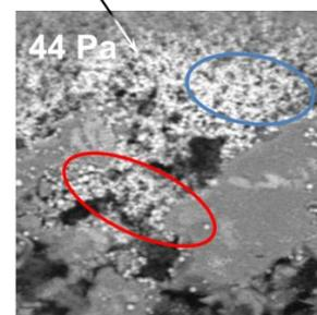
Fig.6 Time-lapse SEM images of cross-sectional views during deposition of TWC particles around surface pores of cordierite GPF substrate
