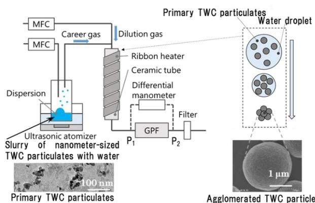
Fig.3 Schematic diagram for fabricating agglomerated TWC particle
