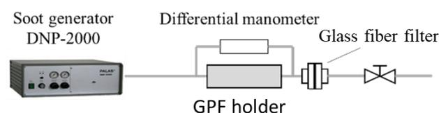
Fig.4 Schematic diagram of setup for soot trapping
