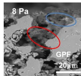
Deposition around necks in surface pores (bridge formation)
