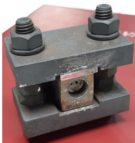
Fig. 2.3 A miniature sample clamped with bolts and nuts setup
