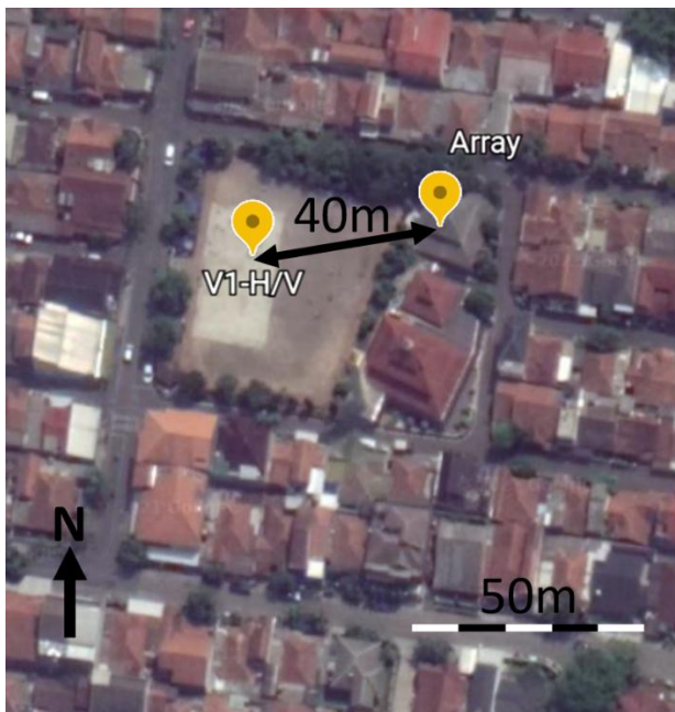
Figure 5.11 Location of the array and the V1-H/V measurement points at S9. The point of the V1-H/V measurement is move 40 m apart from the point of array measurement since a new construction has been built.
