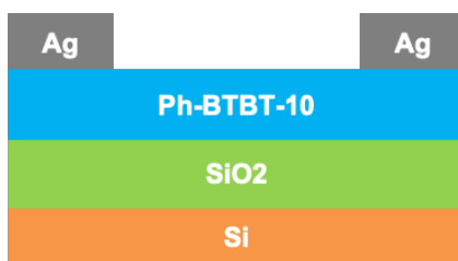
Figure 3.1 Schematic cross-section of Ph-BTBT-10 thin film transistors used in Chapter 3.
