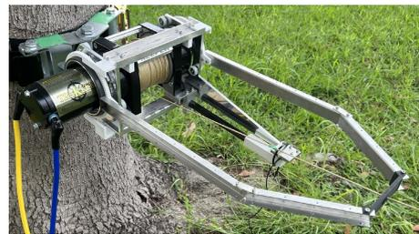
Fig.2 Prototype with tension measurement mechanism.
