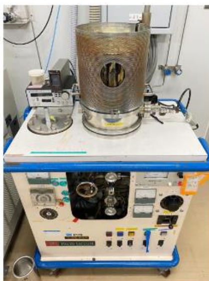
Fig. 3.10 Thermal evaporation system (TOKYO VACUUM, EG-240).
