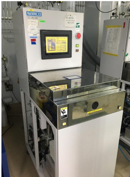
Fig. 3.4 Reactive-ion-etching (RIE) system (RIE-10NR SAMCO)
