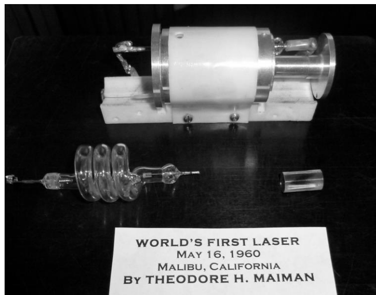
Fig. 1.1 World's first ruby laser designed by T. Mainman [1]
