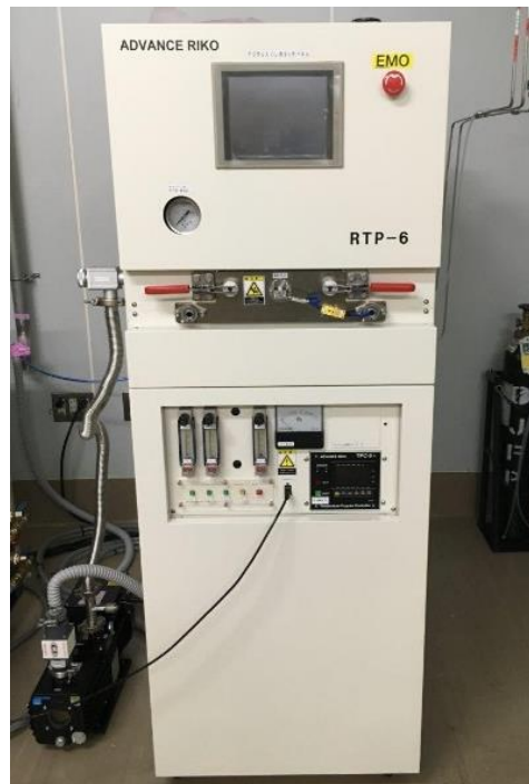
Fig. 3.12 Rapid thermal annealing system (RTP-6, ADVANCE RIKO)
