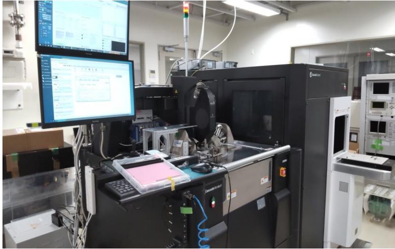
Fig. 3.13 Automated probe system (CM300-Ph, FormFactor)
