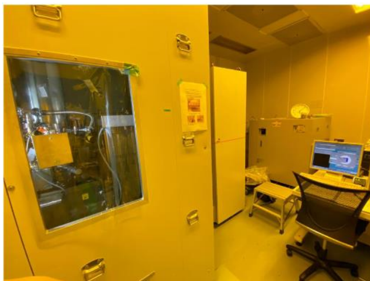
Fig. 3.9 Electron-beam lithography (EBL) system of JEOL JBX-6300FS.
