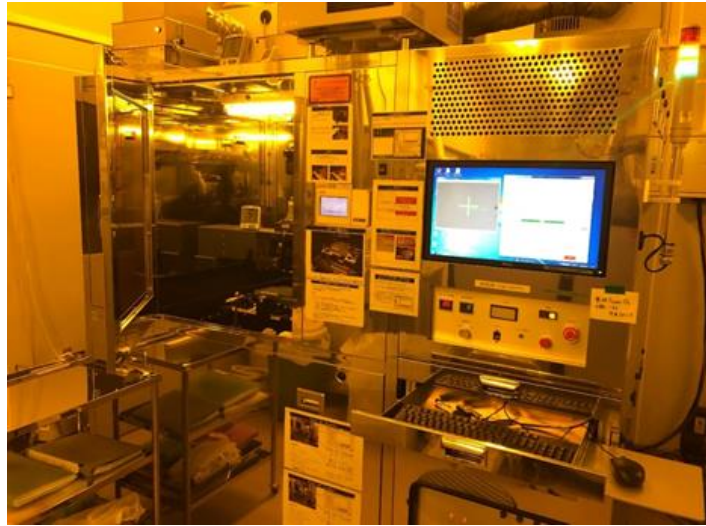
Fig. 3.5 Maskless photolithography system (DNK IP-1007-2(MX-1204))
