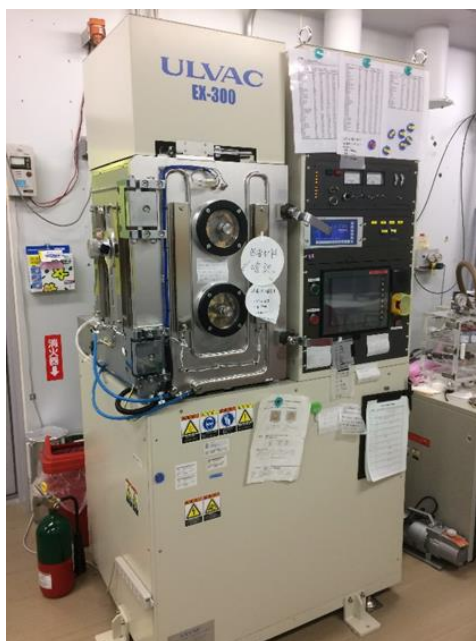
Fig. 3.11 Electron beam evaporation system (ULVAC, EX-300)
