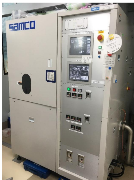
Fig. 3.3 Plasma-enhanced chemical vapor phase deposition (PECVD) system.
