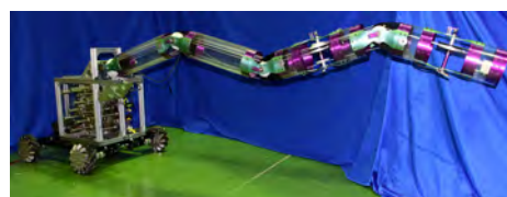
Fig.2 Mini 3D CT-Arm with the fabricated mobile attached.
