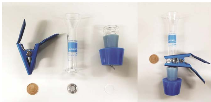
Fig. A.7 Glass mesh holder (Glass Type KG-25, ADVANTEC)
