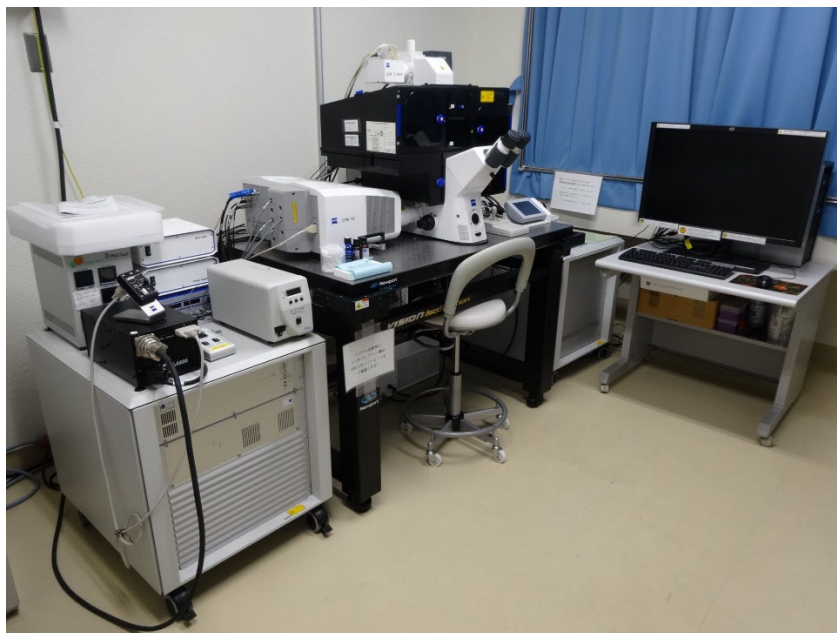
Fig. A.5 Laser scanning confocal microscope (LSM780, Carl Zeiss Microscopy) 1 .
