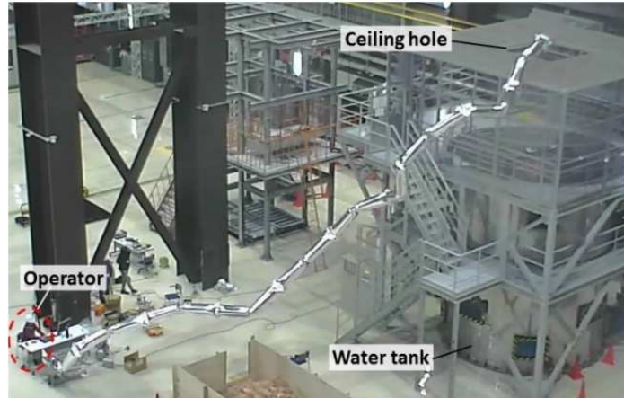
Fig. 1.2 Giacometti arm [36] inspecting the interior of a water tank
