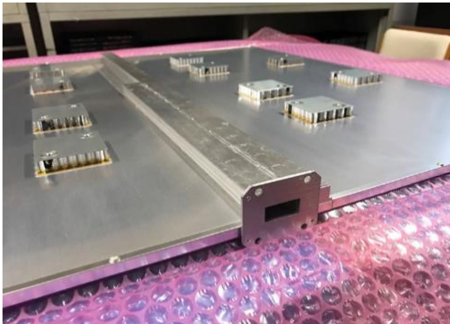
(b) Waveguide feeder mount on the back side of the antenna panel.
