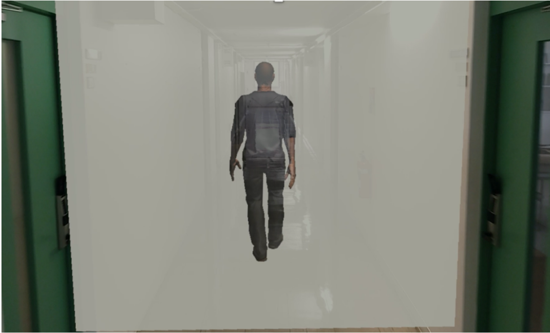
FIGURE 2.5: View of avatar from the head-mounted display. The back of the avatar is observed as the participant walks down the corridor. A translucent white screen is used to make the avatar more visible under bright lighting conditions.
