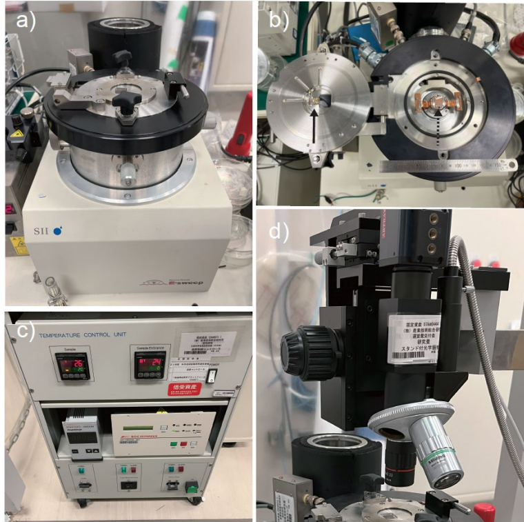
Figure 3.2 The experimental setup for the cohesion force measurement at cryogenic temperatures at AIST. (a) An atomic force microscope (AFM) (SII Nanonavi E-sweep, SII technology Inc.). (b) A cantilever holder and a sample holder indicated solid arrow and dashed arrow, respectively. (c) A temperature controller equipped with AFM and a monitor of a cold cathode gauge (IKR 251, PFEIFFER Inc.). (d) Optical microscopes (MX-51, Olympus Inc.)
