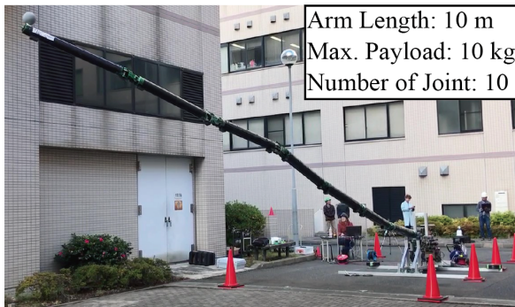
Fig. 3 10 m-long coupled tendon-driven manipulator: Super Dragon
