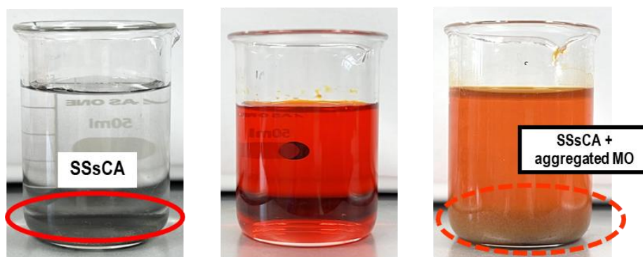
Figure 4.10 Adsorption kinetics of MO adsorption (1000 mg/L) by SSsCA.
