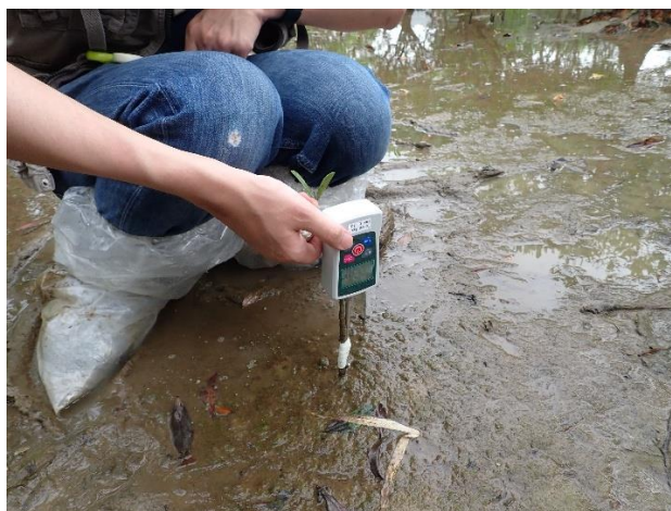
Figure 14. Pulling resistance test of young mangroves using a digital force gauge.
