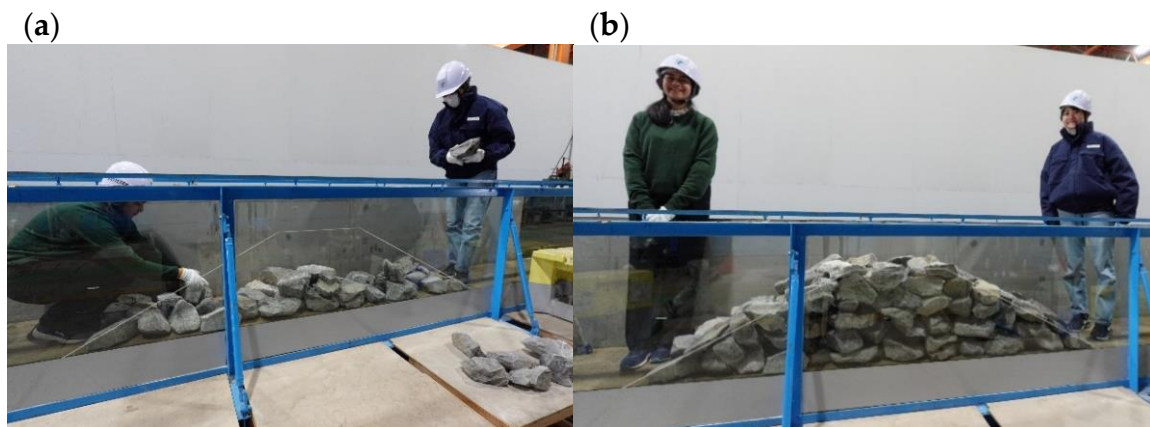
Figure 5. (a) Portable reef being constructed mainly by two female members, and (b) completed reef. Crest height = 0.5 m, crest width = 0.5 m, bottom width = 2.5 m, and side slope = 1:2.
