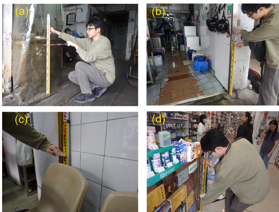
Fig. 2. Inundation depths inside buildings, identified through resident interviews: (a) a port warehouse office, (b) a fish shop, (c) a restaurant, and (d) a pharmacy.
